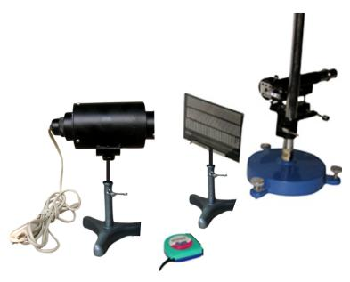
**OMEGA TYPE ES-254** Experimental Set Up has been designed specifically for the Determination of Resolving Power of Telescope. The set-up consists of Telescope, Attachment for Resolving Power of Telescope, board with narrow black & white strips etc.
