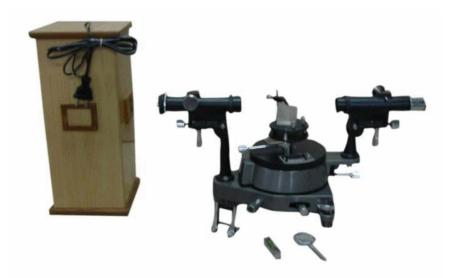
**OMEGA TYPE ES-250** Experimental Set Up has been designed specifically for the Measurement of Refractive Index of glass in the form of prism by Spectrometer. The set-up consists of Spectrometer, Mercury light source, Prism, Reading lens etc.
