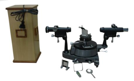
OMEGA TYPE ES-251 Experimental Set Up has been designed specifically for the Measurement of Refractive Index of given liquid using hollow prism by Spectrometer. The set-up consists of Spectrometer, Mercury light source, Prism, Hollow Prism, Reading lens etc.
