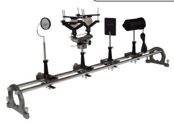
**OMEGA TYPE ES-336** Experimental Set-Up has been designed specifically for determination of Cardinal Points of a system of two thin Convergent Lenses separated by a distance using Nodal Slide Assembly. The set up consists of Optical Bench, Nodal Slide Unit, Light Source, Optical Screen, Plane Mirror and Convex Lenses.
