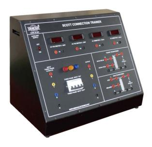
**OMEGA TYPE 20 003** Scott Connections Trainer is an Ideal training board very useful for electrical Labs. It helps in learning Three Phase to Two Phase conversion in a very easy method and to analyse and study the operation of Teaser Transformer and mains Transformer. One can easily perform the experiment and observe the two phase step down wave forms on Oscilloscope having 90° phase displacement with each other.
