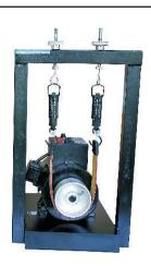
OMEGA TYPE 20 103 DC Machine Lab is a versatile Training system very useful for Labs. It helps to study comprehensively the functioning of DC Motor, Students can perform various experiments including Motor Starting Speed Control, N-I Characteristics etc.
