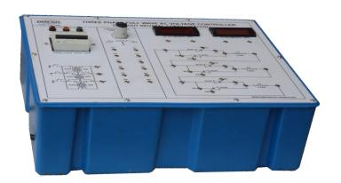
**OMEGA TYPE PET-469** Power Electronic Training Board has been designed specifically for the study of Three phase firing circuit for three phase ac voltage controller (without Neutral Configuration).
