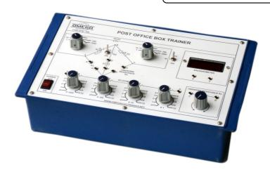
OMEGA TYPE ETB-260 Post Office Box Trainer is the combination of resistances which work on the principle of Wheatstone Bridge. Post Office Box is helpful to determine the unknown resistance of wires like Constantan, and Nichrome etc. With the help of ETB-260 we can determine the specific resistance of different types of wire. Post Office Box can also verify the combination of resistances in series and parallel.
