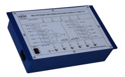
Omega Type LTB-887 Multiplexer and Demultiplexer Trainer has been designed specifically for the study of 4-to-1 Line Multiplexer and 1-to-4 Line Demultiplexer. This Training Board familiarizes the students with the operation of both multiplexer and demultiplexer circuit. It explains the phenomena of Multiplexing of four input signals with two selection lines and one output. It explains Demultiplexing of one input signal with two selection lines and four outputs.
