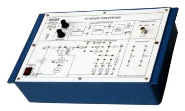
OMEGA TYPE PET-460 is a compact and user friendly learning platform which is very useful for students to understand the concept of PWM generation technique, and Flyback Converter Configuration on various load configurations. It is also helpful for understanding the converter output on various filter configurations. Platform explains PWM generation technique, Flyback Converter Configuration, and power isolation circuit to measure the isolated output.
