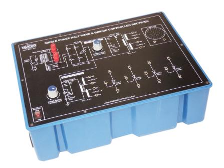
**OMEGA TYPE PET-457** Power Electronic Training Board has been designed specifically to single phase half wave & bridge (Full Wave) controlled rectifier.
