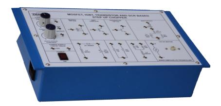
**OMEGA TYPE PET-471** is a learning platform which is very useful for Students to understand the concept of DC to DC chopper on various load configurations. PET-471 is provided with various devices like MOSFET, IGBT, Transistor & SCR.
