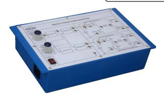
**OMEGA TYPE PET-464** Single Phase PWM Inverter is compact, ready to use experiment board for single phase PWM inverter circuit. This board is useful for students to study and understand operation of single phase PWM firing circuit and single phase PWM bridge inverter using MOSFET/IGBT.
