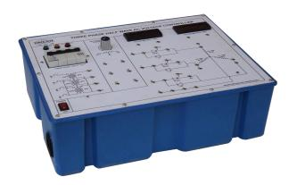
**OMEGA TYPE PET-466** Power Electronic Training Board has been designed specifically for the study of Three phase half wave AC voltage controller drive with Triggering Circuit.
