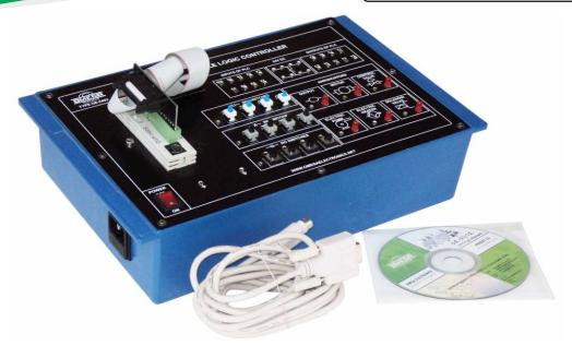
**OMEGA TYPE OE-2402 (PLC,)** is an ideal tool to study the working of PLC's used for industrial applications. has been designed to demonstrate the application of PLC in the area of
