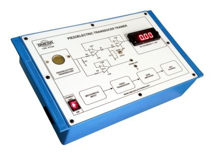
**OMEGA TYPE ICT 929-** Experimental set-up has been designed specifically to study the piezoelectric effect and observe the electrical response generated when mechanical stress is applied to the piezoelectric material. The setup allows hands-on learning of how mechanical energy is converted into electrical energy, offering valuable insight about the working of piezoelectric transducer.
