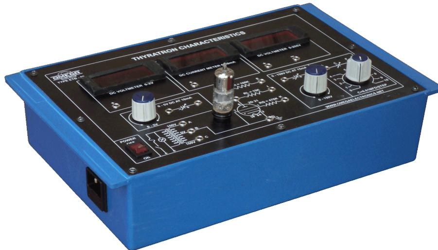
**OMEGA TYPE ETB-80** Experimental Training Board has been designed specifically to study Thyatron Phase, Firing and DC Control characteristics. The unit is absolutely self contained and required no other apparatus.
