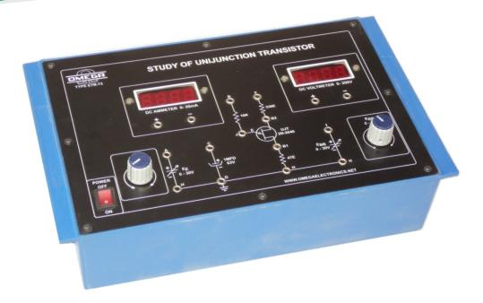
**OMEGA TYPE ETB-73** Experimental Training Board has been designed specifically to study different properties of Unijunction Transistor.
