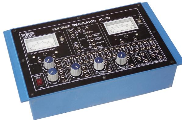
**OMEGA TYPE ETB-86** Experimental Training Board has been designed specifically to study Voltage Regulator IC 723. This Training Board gives a thorough understanding of the basic parameters of IC 723, their measurement and also covers useful applications of this regulator IC. The board is absolutely self contained and requires no other apparatus.
