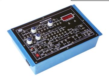
**OMEGA TYPE ETB-95** Experimental Training Board has been designed specifically for the study of Multivibrator circuits. Apart from basic circuits some special techniques have also been included.
