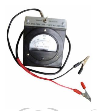
**OMEGA TYPE AF-205** Meters are intended to be used for measurement of A.F. Voltages and Currents. These meters are robust, small in size and have low forward resistance and very low capacitance. These will be very useful in laboratory and radio workshop. These are panel mounting moving coil meters fitted in stands with dial size 65mm. These meters are available in different ranges of Voltages and Currents which are given below.
