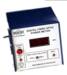
**OMEGA TYPE DFPM-021** Digital-Fibre-Optic Power Meter has been designed with an idea to make available Optic power measurement in the laboratory. It will replace costly Optical Power Meter to facilitate Optic power measurement in dBm.
