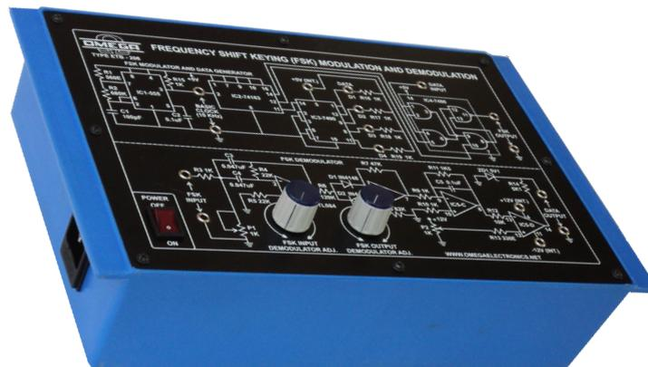
**OMEGA TYPE ETB-206** Experimental Training Board has been designed specifically for the study of frequency shift keying modulation and demodulation.
