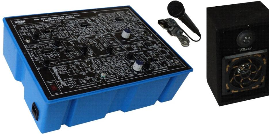
**OMEGA TYPE ETB –232** DSB/SSB-SC Amplitude Modulation & Demodulation Trainer has been designed with a view to provide practical and experimental knowledge of Amplitude Modulation / Demodulation technique as practically implemented in Analog Communication system on a SINGLE P.C.B. of size 300x400mm.
