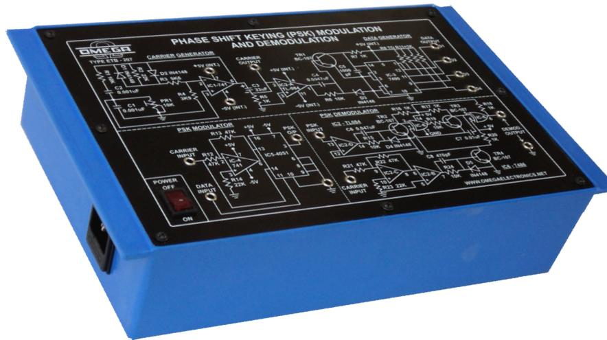
**OMEGA TYPE ETB-207** Experimental Training Board has been designed specifically for the study of the Phase shift keying modulation and demodulation.
