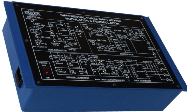
**OMEGA TYPE ETB-222** Experimental Training Board has been designed specifically to study Differential Phase Shift Keying (DPSK) Modulation and Demodulation.
