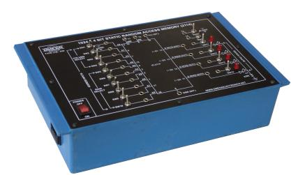
**OMEGA TYPE LTB-830** Computer Logic Training Board on 1024 X 4 Bit Static Random Access Memory (2114) has been designed specifically to get the familiarization and the operation of Semi conductor Memory. It provides the understanding of read, write & chip enable operation with the help of switches and LEDs. Dynamic operation of the chip can also be understood by connecting the pulse generator at the appropriate terminals. The board is absolutely self contained and requires no other apparatus.
