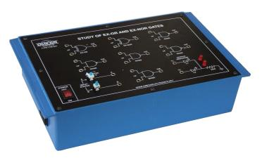
OMEGATYPE LTB-831 Computer Logic Training Board has been designed specifically for the study of EX-OR and EX-NOR Logic Gates and to verify the truth tables of these logic functions using universal NAND Gates. The board is absolutely self contained and requires no other apparatus.
