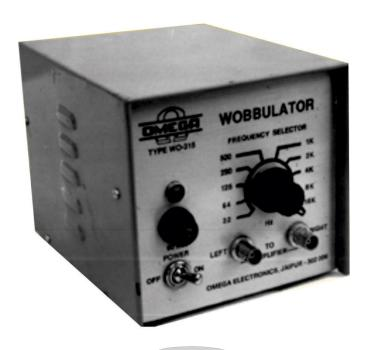
**OMEGA TYPE WO-315** Wobbulator is a Switched Sine Wave Oscillator with ten nominal output frequencies centred on the various octave bands viz. 32Hz, 64Hz, 125Hz, 250Hz, 500Hz, 1KHz, 2KHz, 4KHz, 8KHz, 16KHz. This instrument is very useful for acoustics system i.e. tuning up equaliser etc. The entire unit is housed in a well ventilated sturdy steel cabinet with enamel finish and processed silver grey front panel.
