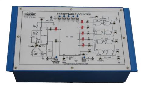
**OMEGA TYPE LTB-835** Computer Logic Training Board has been designed specifically for the study of Presettable Counter. This Training Board gives a better understanding of 5-bit counting, starting from a preset initial number and frequency division of clock input by factors of 2, 3, 4, 5, 6, 7, 8, 9 & 10.
