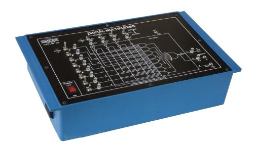
OMEGA TYPE LTB-836 Computer Logic Training Board has been designed specifically for the study of Digital Multiplexer. This Training Board gives a better understanding of the phenomena of multiplexing with eight input signals and one multiplexed output using three control signals. The board is absolutely self contained and requires no other apparatus.
