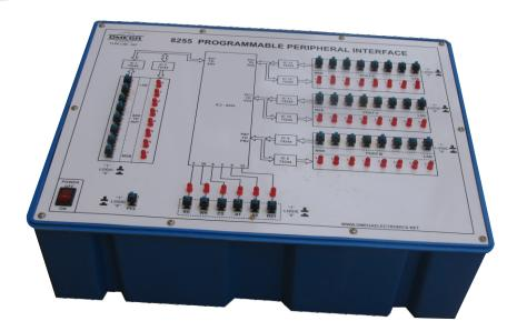
OMEGA TYPE LTB-847 Computer Logic Training Board has been designed specifically for the study of 8255 Programmable Peripheral Interface. This Training Board gives a better understanding of the interfacing between address port & data ports. The board is absolutely self contained and requires no other apparatus.
