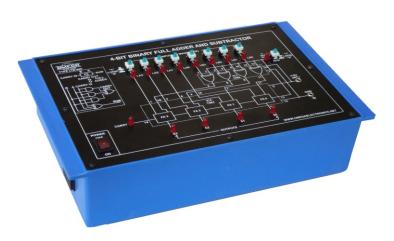
**OMEGA TYPE LTB-860** Computer Logic Training Board has been designed specifically for the study of phenomena of addition and subtraction of 4-bit binary numbers using 4-bit arithmetic and complementary techniques. This Training Board uses controlled inverter and full adders to carry out the operations of addition and subtraction.
