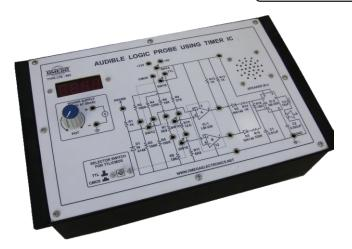
**OMEGA TYPE LTB-862** Computer Logic Training Board has been designed specifically for the study of Audible Logic Probe using Timer IC. It produces a high frequency signal tone when its tip sense high signal, low frequency tone when its tip sense signal is low and a warbling tone (high-low-high...) when encountering a pulse train. This training board gives a better understanding of the concepts involved in construction of Audible Logic Probe and their properties.
