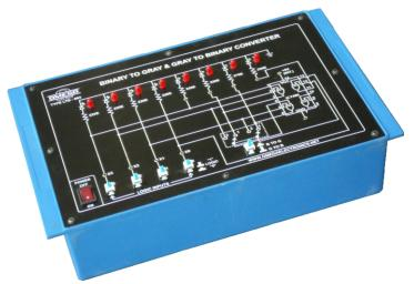
**OMEGA TYPE LTB-863** Computer Logic Training Board has been designed specifically for the study of Binary to Gray & Gray to Binary code conversion.
