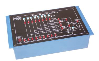
OMEGA TYPE LTB-855 Computer Logic Training Board has been designed specifically for the study of Parity circuits. This Training Board gives a better understanding of checking & generation of Parity. It has 8-bit binary input, one output for checking parity and another 9-bit output with generated odd or even parity.
