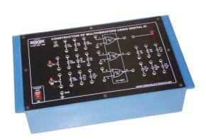
**OMEGA TYPE LTB-858** Computer Logic Training Board has been designed specifically for the study of Bistable, Monostable & Astable multivibrators using digital IC. This Training Board gives a better understanding of the concepts involved in construction of multivibrators and their properties.
