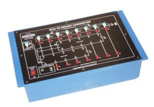
OMEGA TYPE LTB-869 Computer Logic Training Board has been designed specifically for the study of BCD to Binary conversion.
