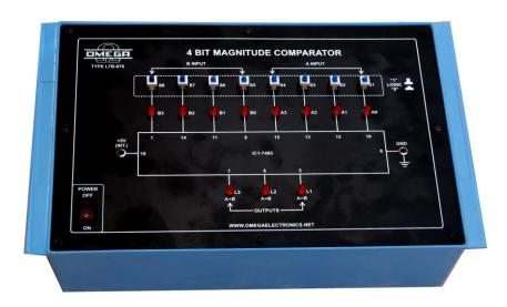
**OMEGA TYPE LTB-870** Computer Logic Training Board has been designed specifically for the study of 4 Bit magnitude comparator (IC 7485).
