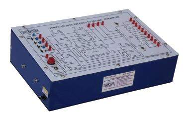
**OMEGA TYPE LTB-867** Computer Logic Training Board has been designed specifically for the verification of Excess-3 to Decimal converter.
