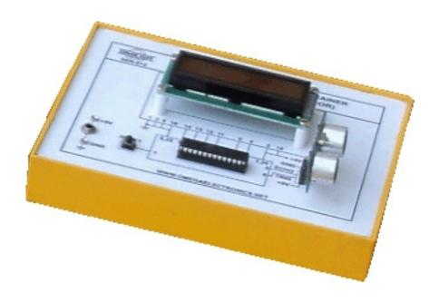
OMEGA TYPE ICT-911 Experimental Set Up has been designed specifically for determining the soil distance of any object or obstacle using Ultrasonic Sensor by the application of ultrasonic waves. The LCD panel directly displays measured distance.
