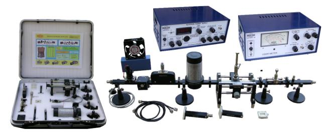
OMEGA TYPE ES-503 uses Klystron tube with its power supply and mount, as a microwave single source along with other standard high quality components and VSWR meter, enables to perform under mentioned experiments. The waveguide components are based on waveguide with plain flanges.
