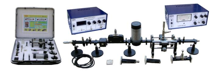
**OMEGA TYPE ES-504** uses low power reflex klystron along with its klystron power supply and klystron mount, as a microwave single source along with other standard high quality components and VSWR meter, enables to perform under mentioned experiments in the laboratory. The waveguide components are based on rectangular waveguide equipped with rectangular plain flanges.
