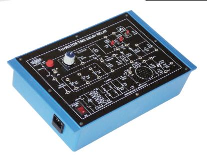
**OMEGA TYPE PET-408** Power Electronic Training Board has been designed specifically to study the operation of SCR and TRIAC triggered by electronic time delay circuit. This facilitates to perform the experiment to students both the modes of operation-delayed turn on and auto turn off to control any type of load i.e.A.C. or D.C.
