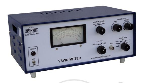
OMEGA TYPE VSWR-796 is a calibrated high gain amplifier to be used for measurement of VSWR, impedance and relative power levels. The meter indicates the signal level in proportion to the input, which is calibrated directly in VSWR and db. This is solid-state version of VSWR meter.
