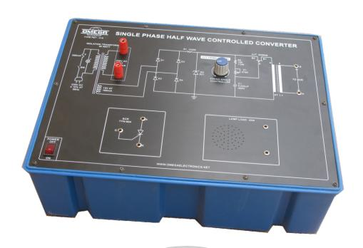
OMEGA TYPE PET-418 Power Electronic Training Board has been designed specifically stydy of single phase half wave controlled converter.
