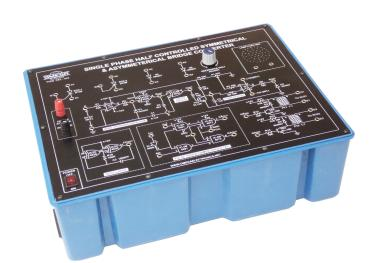
OMEGA TYPE PET-419 Power Electronic Training Board has been designed specifically to study and obtain the waveforms for single phase half controlled symmetrical & asymmetrical bridge converter.
