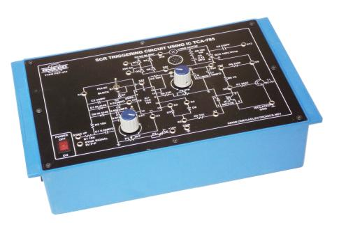
OMEGA TYPE PET-411 Power Electronic Training Board has been designed specifically for the study of SCR Triggering using IC TCA-785. This Training Board gives a better understanding on the operation of Signal Conditioner and Pulse Generator ICTCA-785.
