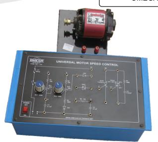
OMEGA TYPE PET-412 Power Electronic Training Board has been designed specifically for the study of speed control of universal motors in different modes, such universal motors are series wound motors capable of operating on both A.C. and D.C. supply. This Training Board is capable of controlling the speed of universal motor up to 1/4th H.P. capacity.
