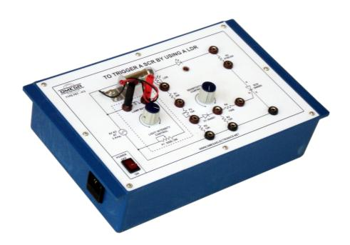
**OMEGA TYPE PET-413** Power Electronic Training Board has been designed specifically to study trigger of a SCR by using a LDR.
